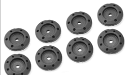
C-00180-768 Shock Piston Heavy Duty - 4mm thick - 8x1.2 + 6x1.4 - 1 Set
